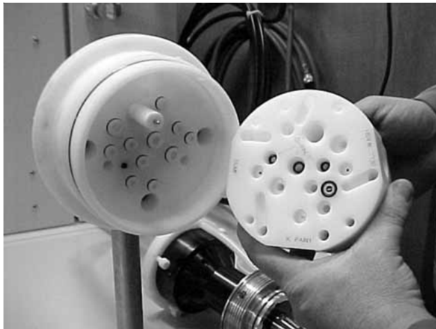
Figure 4: Valve Module Inspection of O-Rings
