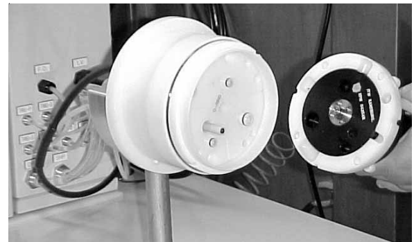
Figure 6: Turbine Assembly Onto the Manifold Assembly
